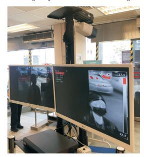
Figure 2 Infrared body temperature screening system located at the main entrance of the hospital.
