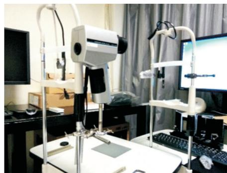
**Figure 1** Gamma correction of the CRT monitor with a luminance meter.
