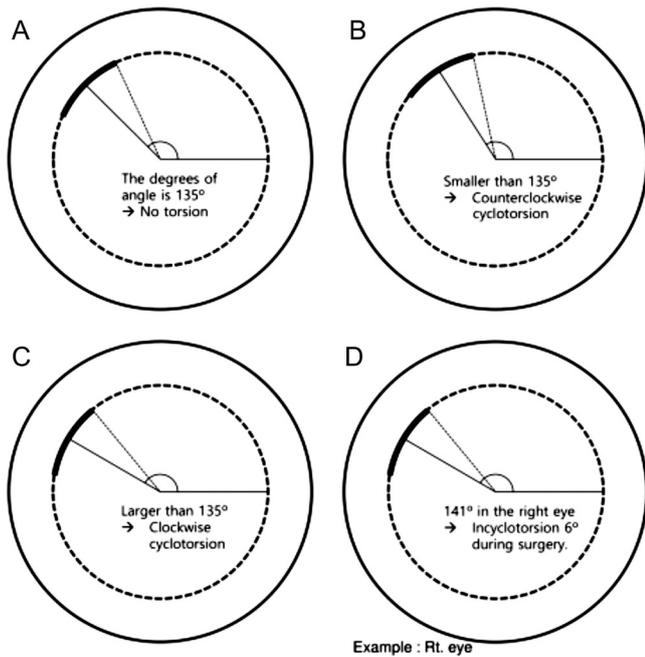
**Figure 2** Cyclotorsion measurement through anterior segment photo analysis after SMILE A: No torsion; B: Counterclockwise cyclotorsion; C: Clockwise rotation; D: Example of the measurement of the right eye incyclotorted. SMILE: Small incision lenticule extraction.
