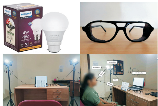
Figure 1 Experimental setup, including light used and wraparound spectacle frame with blue light blocking lenses (BBL).
