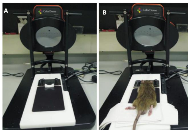
**Figure 1 Experimental setup** A: ColorDome Ganzfeld System (Diagnosys, Lowell, MA, USA); B: The animals were placed black heating pad and connected with electrodes.
